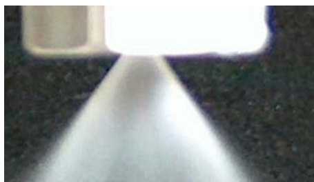
Fig A.3 Spray cone, pressure drop 7 bar.
