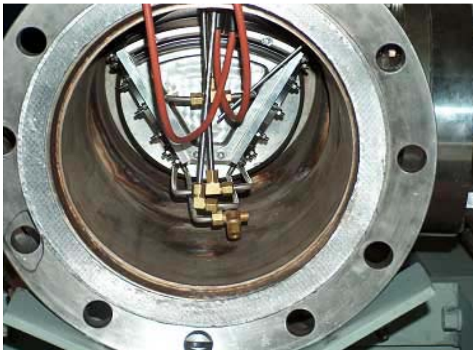
Fig 1.8 Combustor sector assembled within test rig, piping connections.
