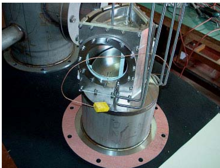
Fig 1.4 The assembled combustor sector, mounted on the interface section to the Combustor test rig.
