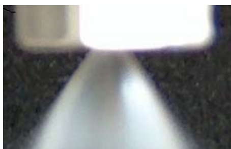
Fig A.2 Spray cone, pressure drop 2 bar
