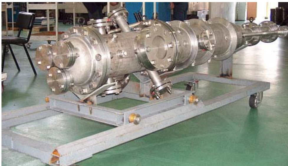
Fig 1.6 Main structure of the combustor test rig, complete and hydrostatically tested for 12 bars
