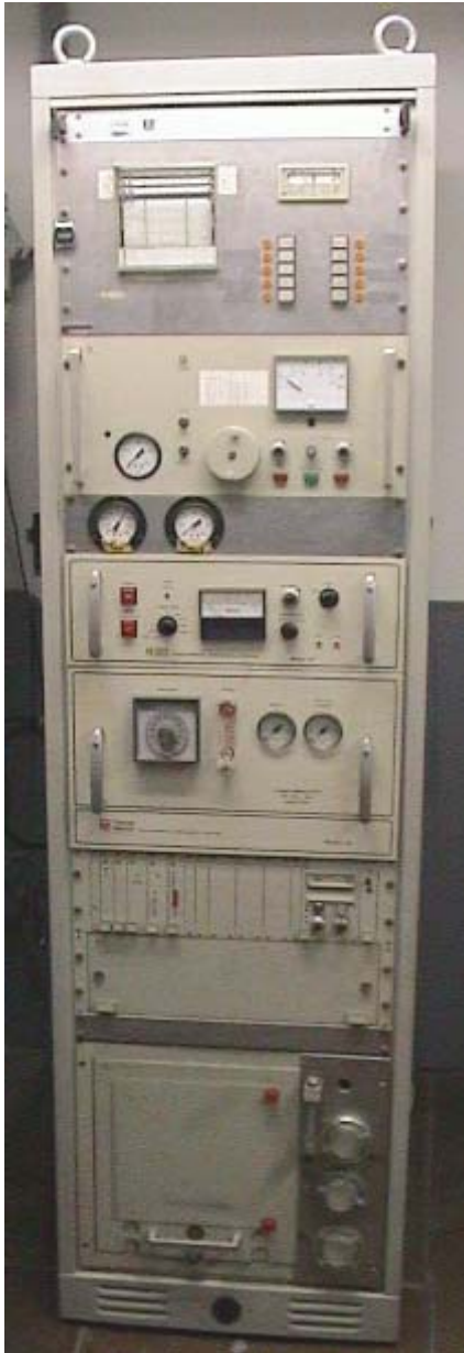
Fig 8.12 Exhaust gas analyze system CO, CO 2 , NO x , HC
