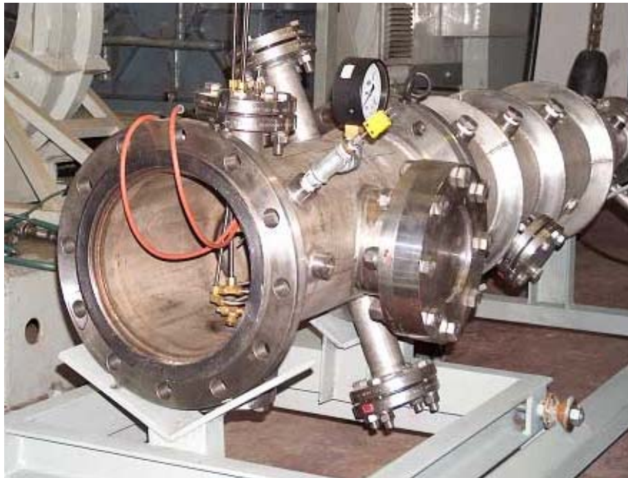
Fig 1.7 Combustor sector assembled within test rig.
