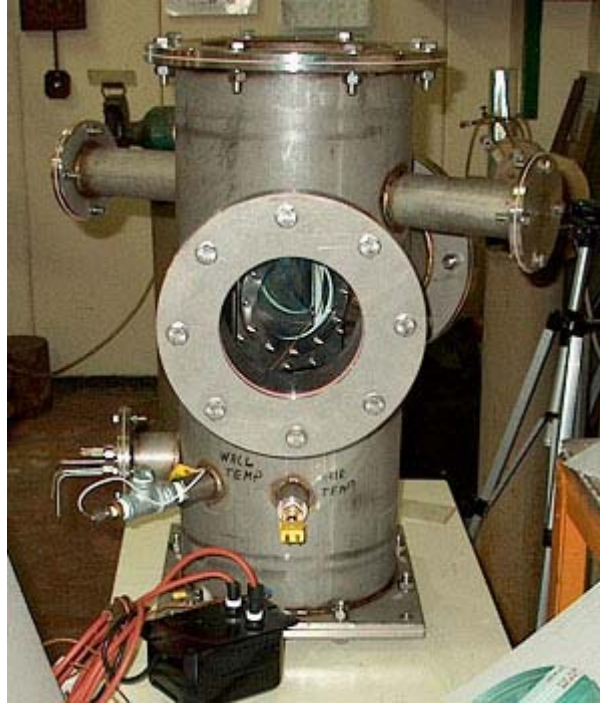
Fig 1.3 The combustor sector test rig, assembled and incorporating the combustor sector.
