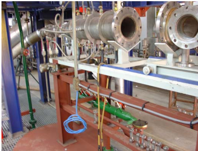
Fig 6.1 Pressurised test rig. Detail of discharge section (left) and air inlet tubes (right)
