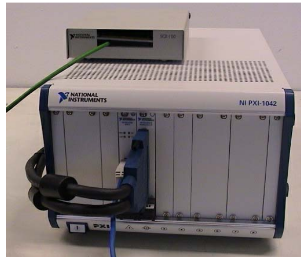
Fig 8.15 Data acquisition unit
