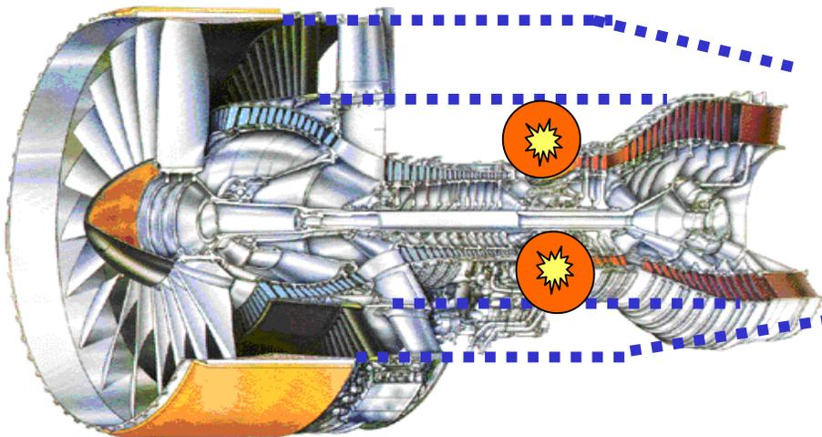
$$\frac{U_{9'}^2}{2} = \eta_n C_{pc} T_{07'} \left[ 1 - \left( \frac{P_{9'}}{P_{07'}} \right)^{\frac{\gamma_c - 1}{\gamma_c}} \right]$$
